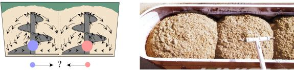
One must ensures that concentrates are distributed evenly in the mixer on these machines to obtain the best mixing results and not fill them all in one end of the machine.
