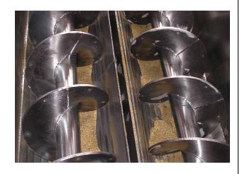
The Cormall MTX mixer can be delivered with extra teight small distance between the auger and the mixer bottom, thus leaving as little leftover from previous mix as possible
