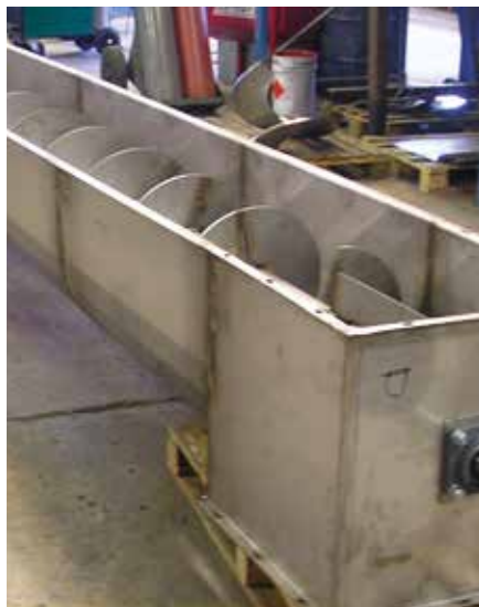
AISI 316 L, conveying auger for transport of acid material.
