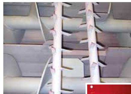
MTX_A agitator device for homogenizing straw mixed with molasses, removes the lumps.
