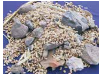
Above picture shows the normal contamination's found in our pneumatic stone trap.
